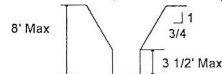
Figure 3. Type A Soil Unsupported, Vertically Sided Lower Portion, Max 8 Feet in Depth
